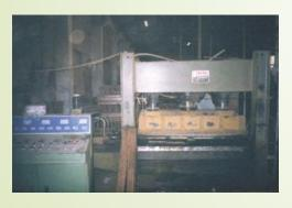
4. Units are pressed together in a hot press to form floorboards
