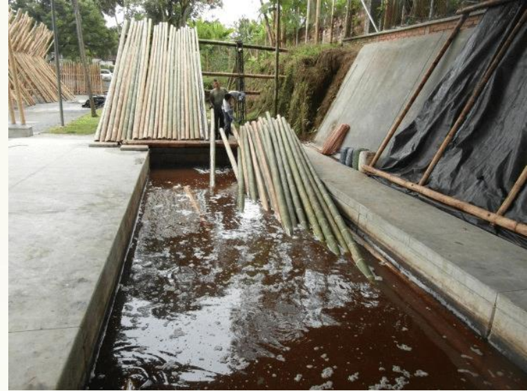
Bamboo Treatment by dipping process
