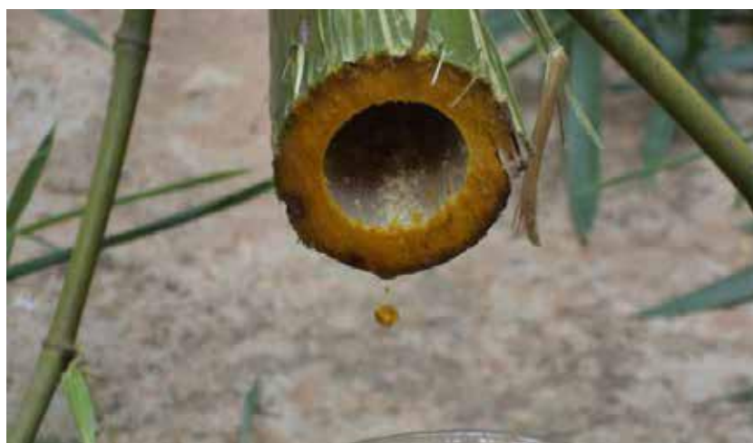
Dripping of preservative
