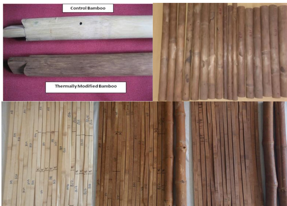
Fig.3 Thermally modified bamboo round bamboo and strips
