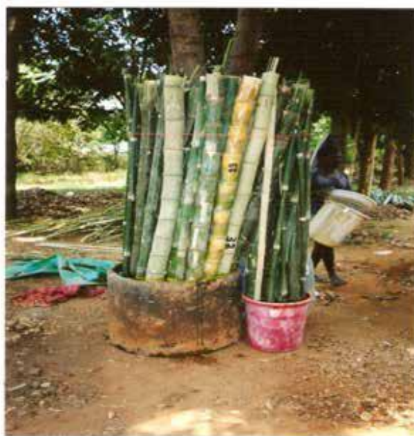
Green Bamboo immersed in preservative solution
