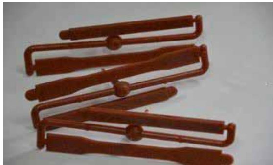
Fig. 6: Test specimen for evaluation of mechanical properties of WPC
